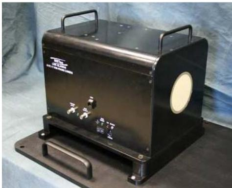
Figure 1: NSTec's VarFrame camera has a variable frame count of 1 to 25 frames at 6.6 million frames per second
