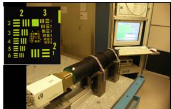
Figure 3. CCD calibration laboratory for flat field, dynamic range, spectral response, and sensitivity measurements
