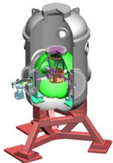
Figure 2. – The Dual-Axis Confinement System (DACs). The green vessel is a 6' diameter blast confinement vessel. The gray vessel provides containment of hazardous materials, and radiation shielding. The experiment is aligned using the orange basket.
