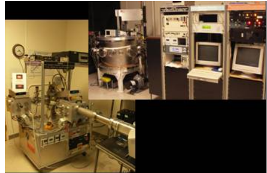
Figure 2. X-ray laboratory for x-ray streak camera, x-ray gated imager, and x-ray component characterization
