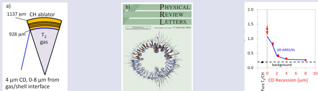
Figure 1. a) Schematic of the CD Symcap capsule. The capsules are filled with pure tritium gas and contain deuterated plastic layers at various distances from the gas/shell interface. b) ARES simulation of a CD symcap implosion, featured on the January 2014 cover of Physical Review Letters, showing the mix of D from the plastic ablator with the T gas core. c) Measured DT to TT neutron yield ratio for CD Symcaps, as a function of the recession depth for the CD layer from the gas/shell interface. The DT/TT yield ratio, a measure of the atomic mix in the core, decreases as a function of recession depth demonstrating sensitivity of the platform to gas/shell mix. Results from ARES simulations are also compared to the observations.
