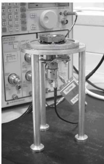
Figure 14. GHz Ultrasonic interferometry DAC technique. Compressional and shear-wave travel times down to \sim 10 nanoseconds in duration can be measured on dense, opaque materials with a nominal accuracy of a few parts in a thousand. Compressional waves with 5\text{-}10\ \mu\text{m} wavelengths are produced at a sputtered ZnO thin-film transducer. Purely-polarized shear waves are generated by P-to-S conversion upon reflection inside an acoustic buffer rod 92 .
