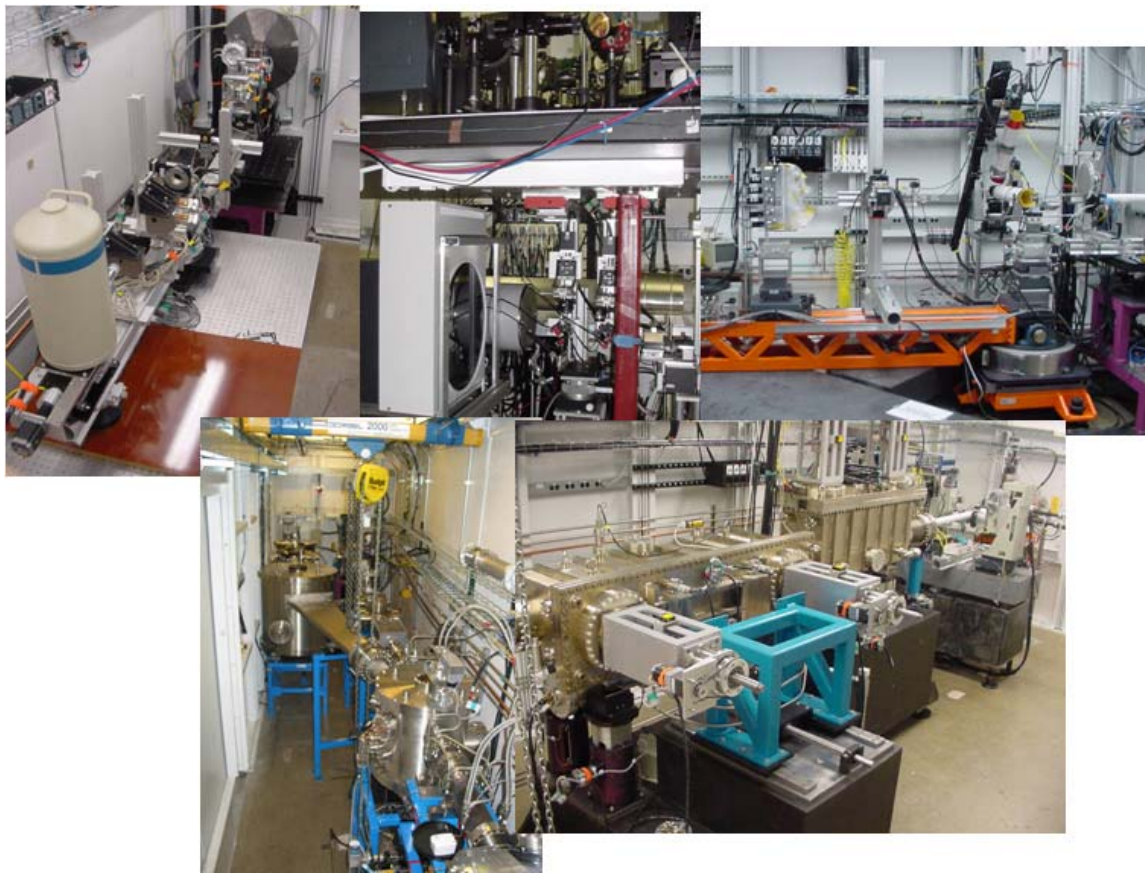
Figure 35. Clockwise from top left: The construction of a diffractometer in 16BM-D; the x-ray diffraction station at 16ID-B of HPCAT provides state of the art techniques, including micro-focused beam, area CCD and image plate detectors, and in-situ double-side laser heating, for high-pressure and high-temperature x-ray diffraction studies; the setup in 16ID-D. The NFS, XRS, RXRS, and XES have been successfully commissioned in ID-D, and will become operational in 2006; the setup in 16ID-D. The NFS, XRS, RXRS, and XES have been successfully commissioned in ID-D, and will become operational in 2006; the BDCM monochromator installed in 16ID-A, allowing single undulator beam to be split into two branches: one for spectroscopy experiments at 16ID-D station, and the other for micro-diffraction experiments at 16ID-B. The BDCM is a horizontally deflecting monochromator delivering beam to the ID-B station. Si<220> crystals are mounted in the monochromator and the energy range is 24 keV to 35 keV. The crystals are water cooled. The horizontal offset from the main beam is 1 meter outboard. Bimorph mirrors focus the beam to 15 \mu\text{m} X 10 \mu\text{m} in the ID-B station.
