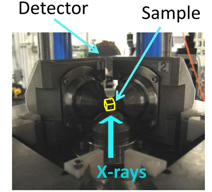
Samples were deformed in the D-DIA at APS. Sintered cylinders of various volume fractions of the two phases were compressed then stressed uniaxially. Diffraction patterns were collected *in situ* up to approximately 4 GPa, 800°C, and 50% strain in order to observe evolution of preferred orientation.
