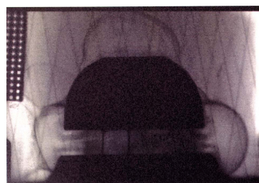
Figure 2. Data from the Features II experiments on Z acquired by imaging a radiation driven, hydrodynamic shock. Measurements of the shock position along the axial and radial axis directly relate to the delivered energy and subsequent radiation flow.
