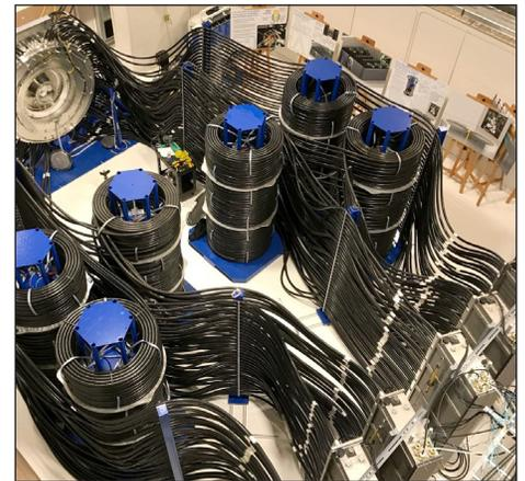
An overhead view of Thor 48 with six brick towers, six cable towers, and the load region. (Photo by Brian Stoltzfus)
