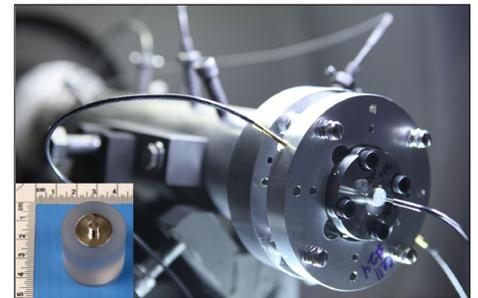
A pre-compressed hydrogen-helium target mounted on a two stage light gas gun in preparation for a dynamic compression experiment at Sandia National Laboratories. Inset - platinum impactor mounted on a projectile for the gas gun. The projectile was launched into the target at five kilometers per second. (Photo by Bernardo Farfan)
