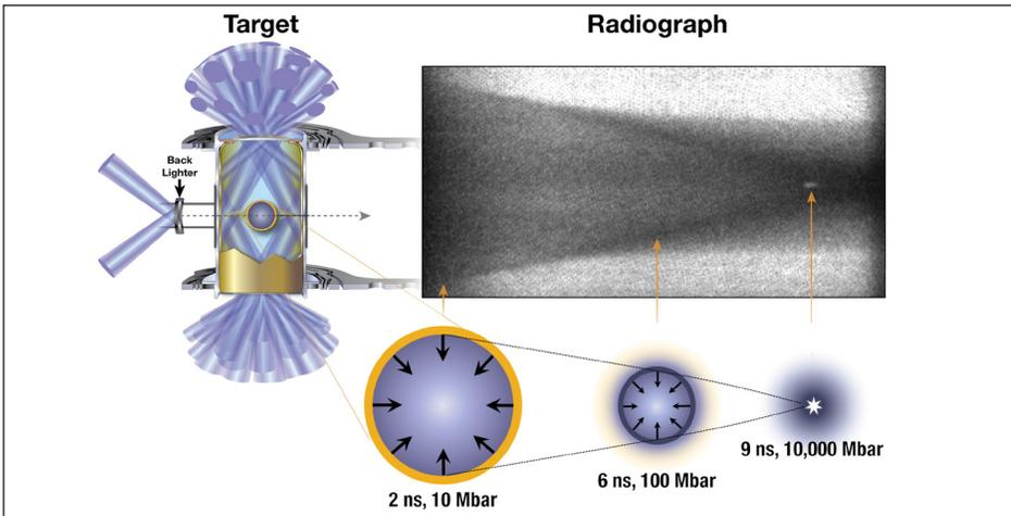
Figure 2. The NIF Gbar shock platform uses a hohlraum to drive a solid sphere and a backlighter to image the imploding sphere onto a streak camera through narrow slits in the hohlraum. The streak camera radiograph records the position of the converging shock front from the time when it passes from an ablator layer into the sphere until coalescence, where x-ray self-emission from the hot spot is evident.
