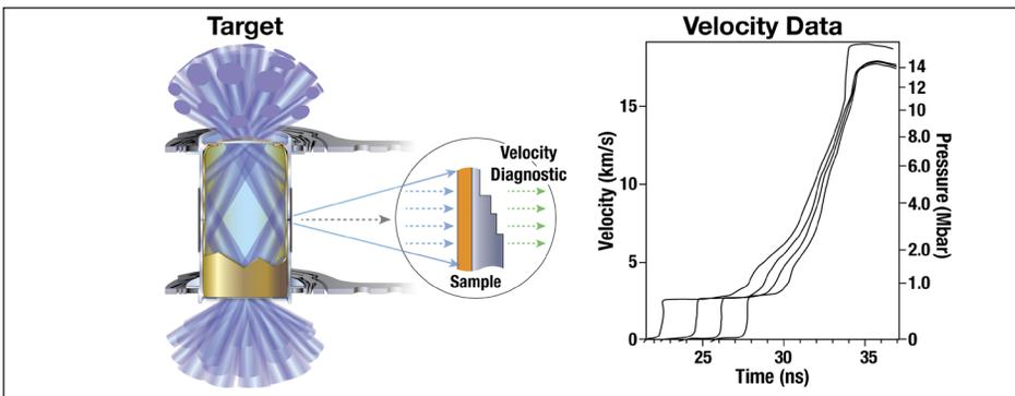
Figure 3. The NIF Ramp platform utilizes a hohlraum target with a stepped sample mounted on the side. In these experiments, a velocity diagnostic measures compression wave steepening as a function of material thickness. By measuring the wave steepening for different sample thicknesses, we determine the material sound speed and ultimately the sample pressure and density response.
