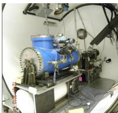
Figure 2. The removable JASPER Primary Target Chamber (PTC) (blue) is located inside the Secondary Containment Chamber (white). The high-velocity projectile enters through the front of both chambers and shocks a Pu sample inside the PTC.
