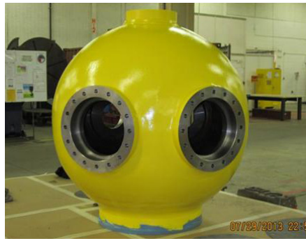
Figure 5. Three-foot-diameter subcritical experiment spherical confinement chamber showing radiographic ports (side) and diagnostic feedthrough cover (top).
