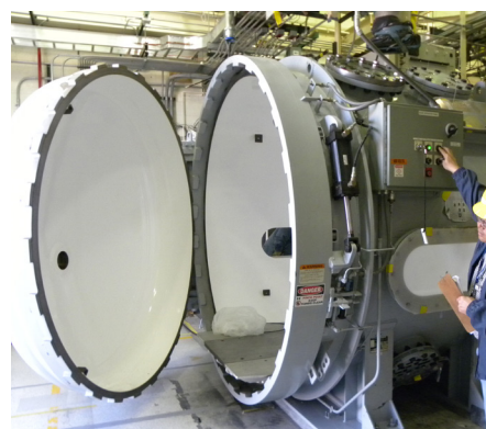
Figure 3. The JASPER Secondary Containment Chamber provides the infrastructure for supporting samples and experiments inside the PTC, including diagnostic feedthroughs, vacuum ports, x-ray ports, and trigger and timing systems access.
