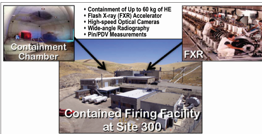
Figure 2. The Containment Chamber and the FXR at the Contained Firing Facility at LLNL's Site 300.
