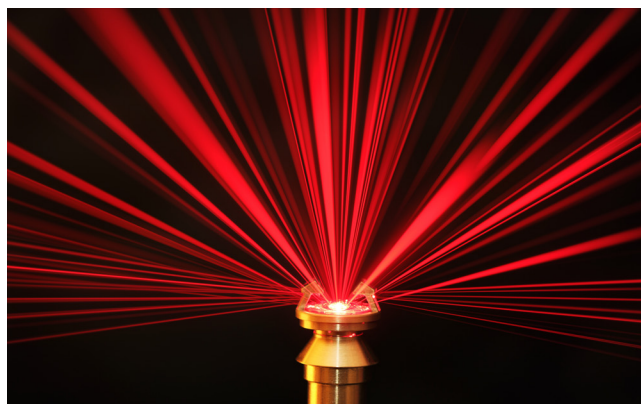
Figure 3. A multiplexed PDV probe used to record the velocity of pit surface during the implosion.
