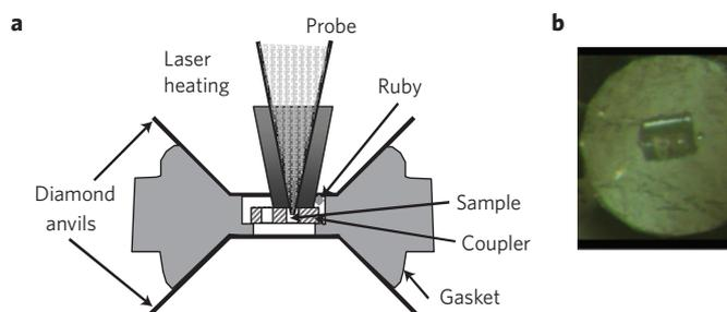
**Figure 1 | Laser-heating experiment.** **a**, Schematic diagram of the sample arrangement in a DAC cavity. **b**, Microphotograph of a DAC cavity before heating.
