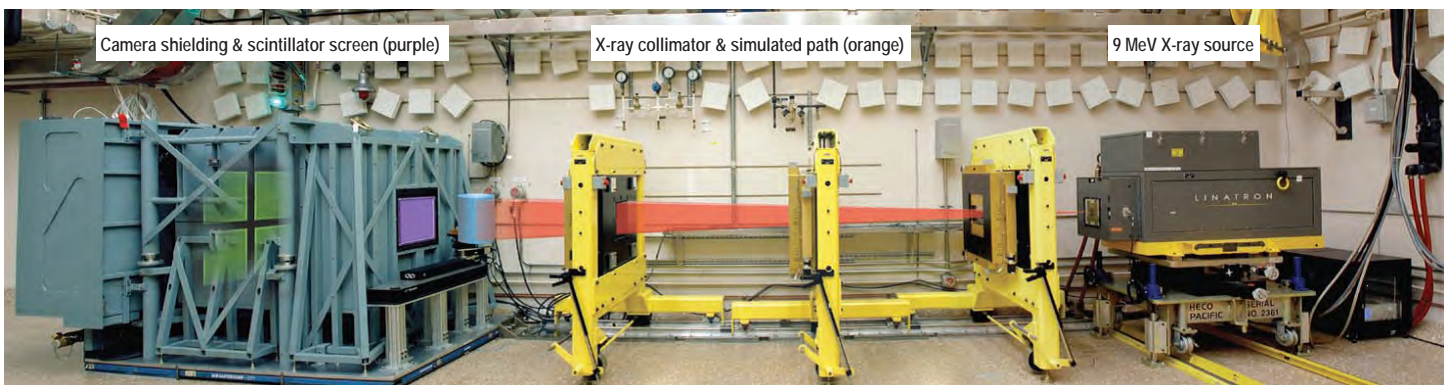
Figure 3. The CoLOSSIS (Confined Large Optical Scintillator Screen & Imaging System) X-ray CT system at DOE/NNSA's Pantex Plant is dramatically increasing the inspection rate for pits. A second unit is being planned to meet future demand.
