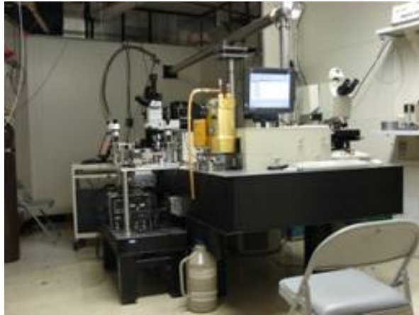
Fully upgraded U2A end station with new Raman systems
