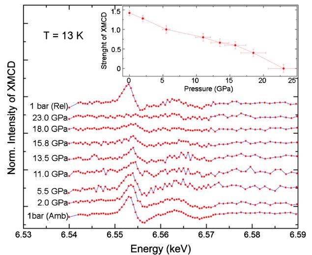
FIG. 2 (color online). Normalized XMCD data of manganite  $\text{La}_{0.75}\text{Ca}_{0.25}\text{MnO}_3$  collected at 13 K from 1 bar to 23.0 GPa. The inset shows the intensity of overall XMCD strength versus pressure. [“1 bar (Rel)” is taken after pressure release; “1 bar (Amb)” is taken at ambient conditions].
