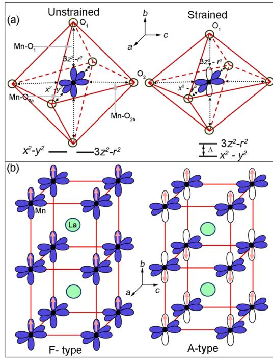
FIG. 4 (color online). (a)  $MnO_6$  octahedra at unstrained and strained conditions. The filled  $e_g$  orbitals are occupied by electrons, while the opened  $e_g$  orbitals are not occupied by electrons; (b) the structure models for *F*-type and *A*-type magnetic ordering. The arrows inside orbitals indicate the spin direction of  $d$  electrons.
