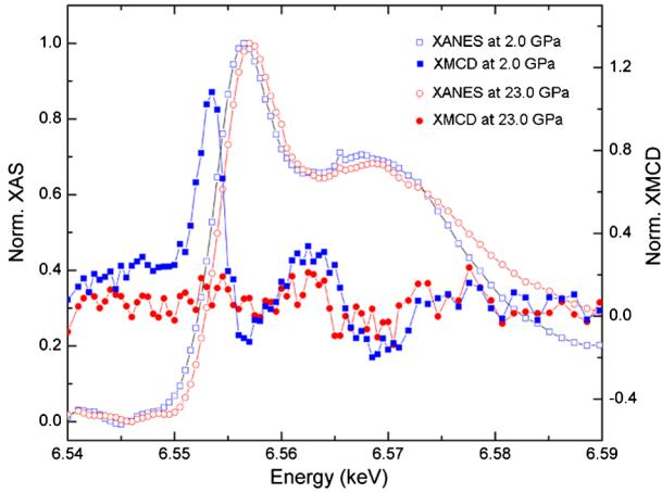
FIG. 1 (color online). Normalized XANES and XMCD data for  $\text{La}_{0.75}\text{Ca}_{0.25}\text{MnO}_3$  at 13 K collected at 2.0 and 23.0 GPa. The XMCD peak intensity is about 0.1% of the absorption jump.
