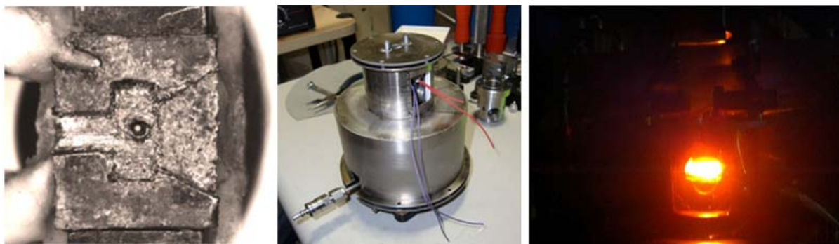
Figure 35. Left: Graphite heater within a DAC. Center: Resistive heating assembly with DAC cell set up inside and thermocouples attached. Right: Fe-Ni alloy sample at 2000 K inside a DAC.
