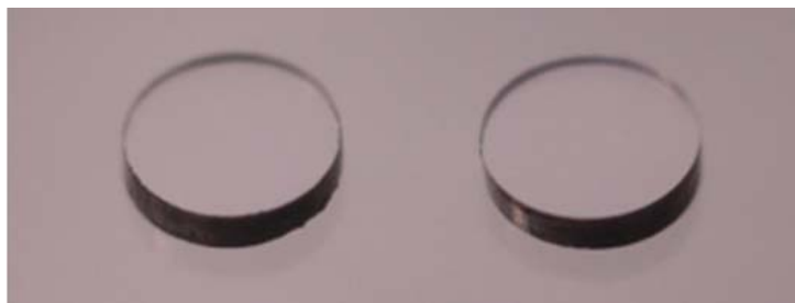
Figure 67. Single crystal CVD diamond windows for small angle x-ray scattering studies at high pressure. Windows are 3.0 mm in diameter and 0.5 mm thick.
