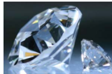
Figure 83. Above: 2.3 ct colorless single crystal CVD diamond anvil compared to a 0.25 ct anvil. Left: UV-VIS transmittance and PL/Raman spectra (excited by 457nm laser) of the 2.3 ct CVD diamond anvil, the inset shows the second-order Raman peak.
