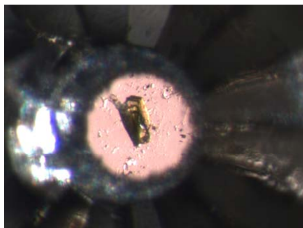
Figure 1. (Left) Photomicrograph of a single crystal of TATB in a diamond-anvil high-pressure cell; (Right) Single-crystal diffraction pattern for one orientation of this sample
