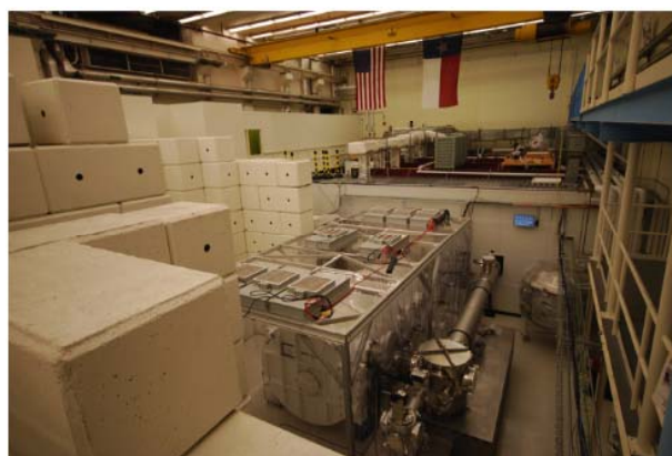
Figure 2. Photo of the target bay of the Texas Petawatt showing the white vacuum tank housing the pulse compressor at the target chamber which is devoted to the fusion neutron generation experiments
