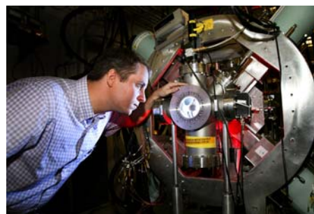
Figure 3. Rutgers postdoc William Peters inspects the detectors used in the neutron capture surrogate reaction study with arsenic beams
