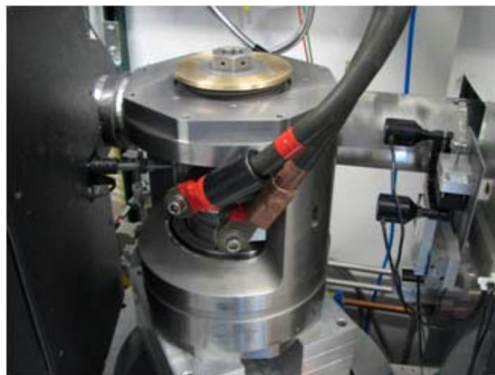
Figure 77. In-situ heating experimental setup. A custom-made precision collimator is applied to obtain a high signal to background ratio, which is one of the key challenges, especially for low-Z and non-crystalline materials. We expect this PEC setup at 16-BM-B will bring more opportunities to study materials properties and phase transitions in amorphous and liquid materials and oxide/silicate minerals under high pressure and temperature, which will be complementary to DAC measurements.
