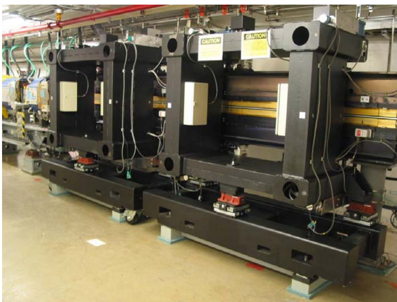
Figure 73. Dual undulators installed in tandem mode on beamline 16-ID at HPCAT.
