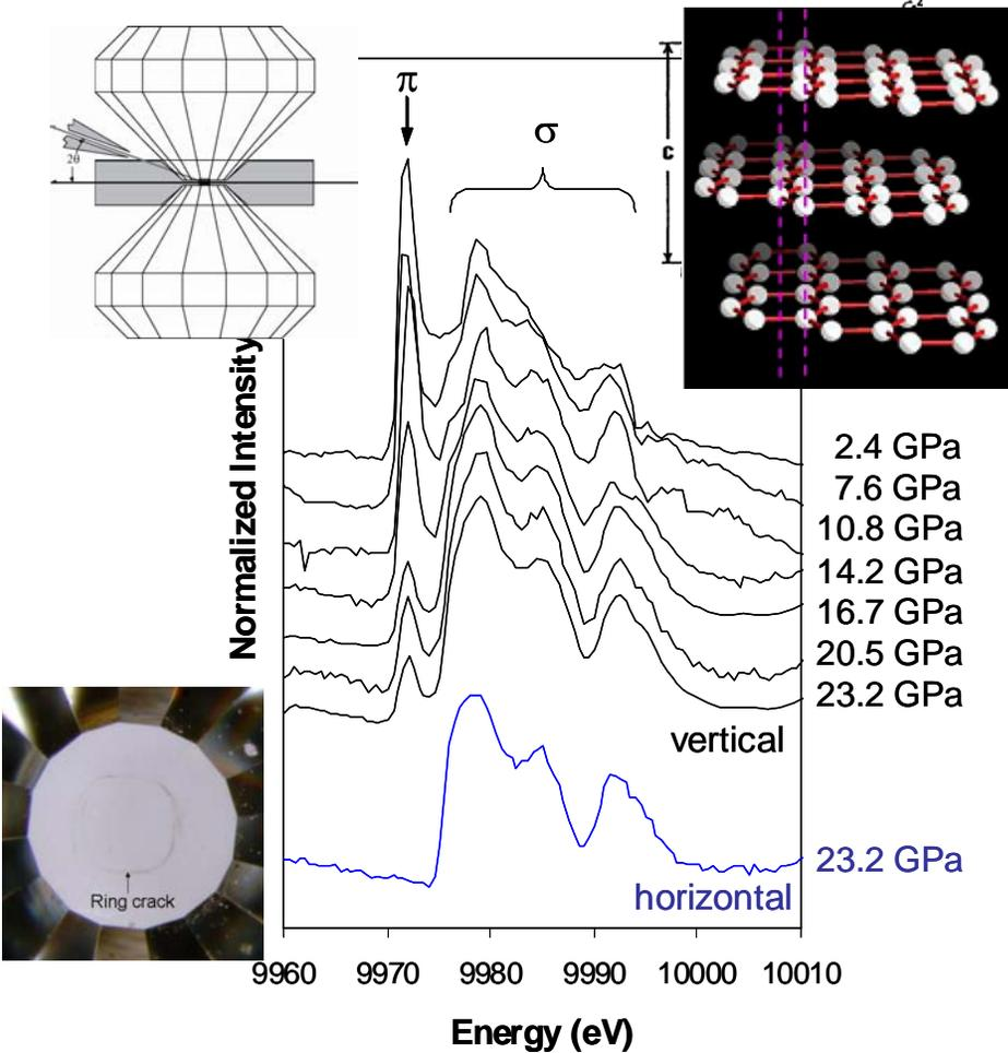
X-ray raman of graphite at high pressure showing the evolution of bonding and transformation to a new, superhard phase
